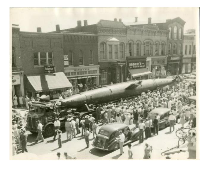
The naval engineers had spent some time studying the sub and then allowed it to be used for exhibition. As originally equipped, the sub weighed between 32 and 35 tons. Before being used for display, the mechanical equipment was removed reducing the weight to about 17.5 tons.
